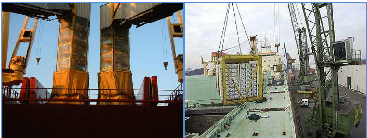
Banana handling technology for reefer vessels: spiral conveyor system for individual boxes (left) and pallet cage (right)
