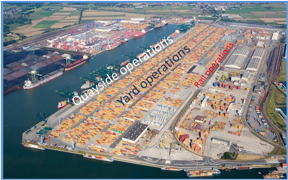
Modal separation at a container terminal (MSC Home Terminal in Antwerp)
