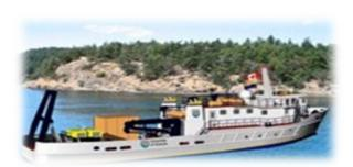
for fisheries patrol and maintenance) with new green ship technology to become the world's first plug-in hybrid "green ship" powered by electricity, hydrogen fuel cells and low-emission diesel fuel. It will come in service by late 2012.
