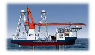
**Beluga- Hochtief**: A heavy- lift, jack- up vessel for use in the offshore wind turbine market. Mainly to be used in offshore construction market, the first vessel will be employed in the Global tech I Offshore Wind Farm. The entry of this vessel is said to address the problem of onerous offshore
